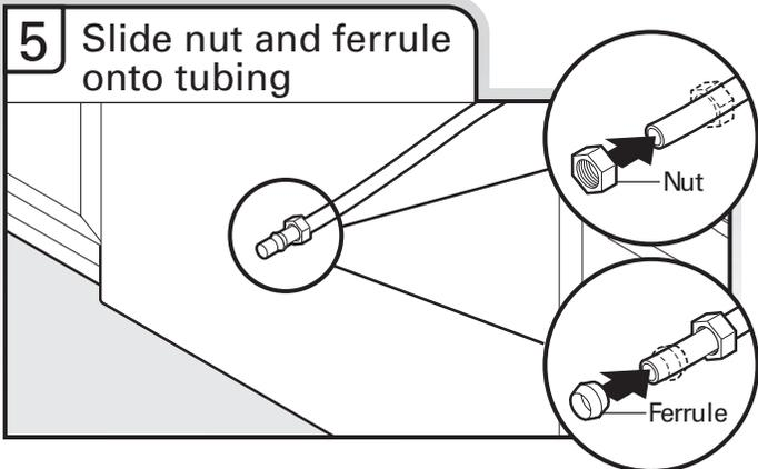
Copper tubing only: Slide nut, then ferrule, about 1" (2.5 cm) onto copper tubing.
